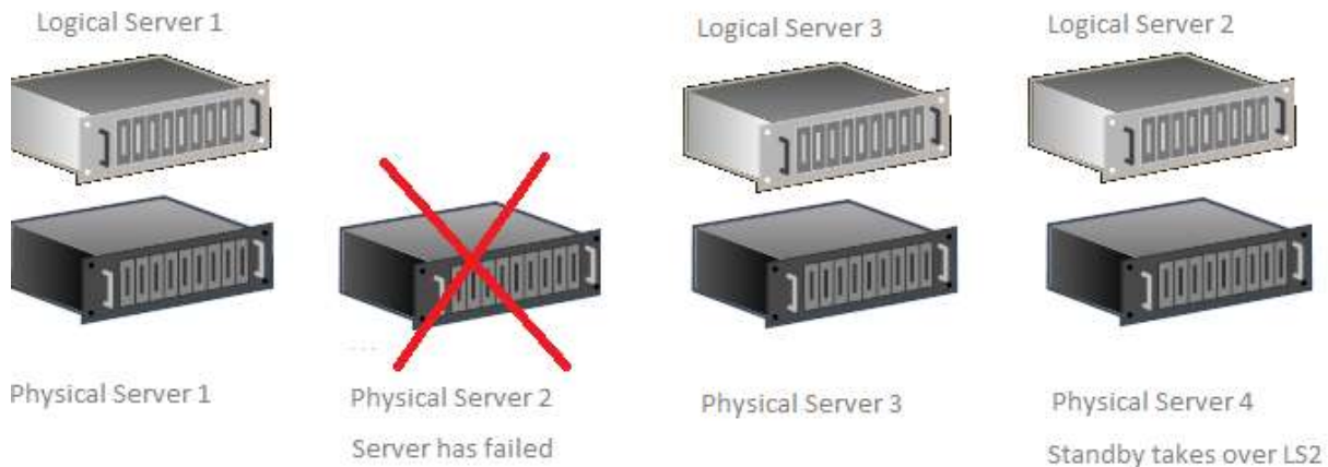
Figure 11.14: Failover logical and physical devices after failure
