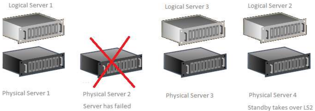
Figure 9.14: Failover logical and physical devices after failure
