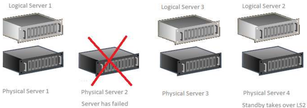
Figure 9.15: Failover logical and physical devices after failure
